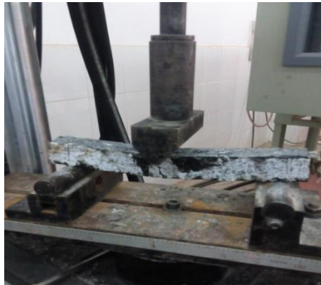
Fig.1 Mts Three-Point Bending and Drawing of Material Test System
